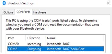
• To access the serial interface, the COM port with the direction Outgoing and the designation SerialPort must be used.
